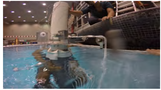
Fig. 11 1:50-scale prototype upper platform during pool testing.
