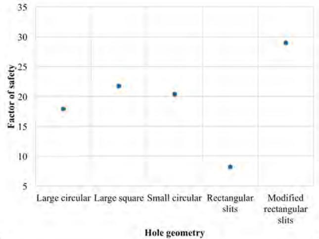
Fig. 6. Factor of safety as a function of hole geometry for the cube shell enclosure.
