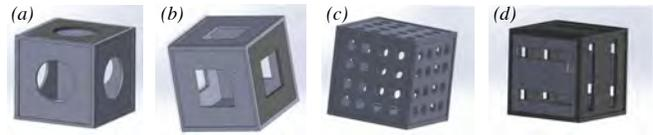
Fig. 5. Solid models depicting cube shell enclosure with (a) large circular, (b) large square, (c) small circular, (d) rectangular slit hole geometries.
