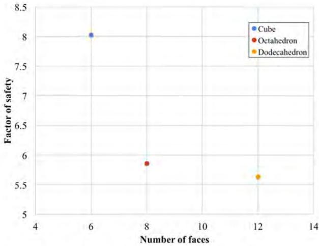
Fig. 4. Factor of safety as a function of number of faces for the dodecahedron, octahedron, and cube shell enclosures.
